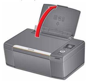
2. Open the output tray, then pull out the extender until it is fully extended.
