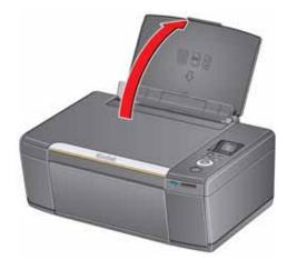
2. Pull out the output tray until it is fully extended.
