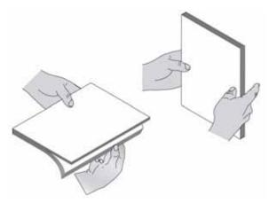
2. Make sure the left and right paper-edge guides are in the plain-paper position, then insert the paper into the input tray.
