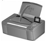
**2** Pull out the output tray until it is fully extended.
