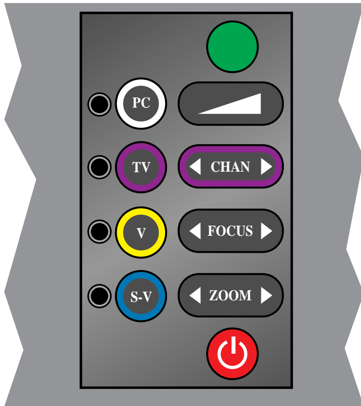
Figure 14: The keys on the touch panel on the KODAK DP850 ULTRA projector
