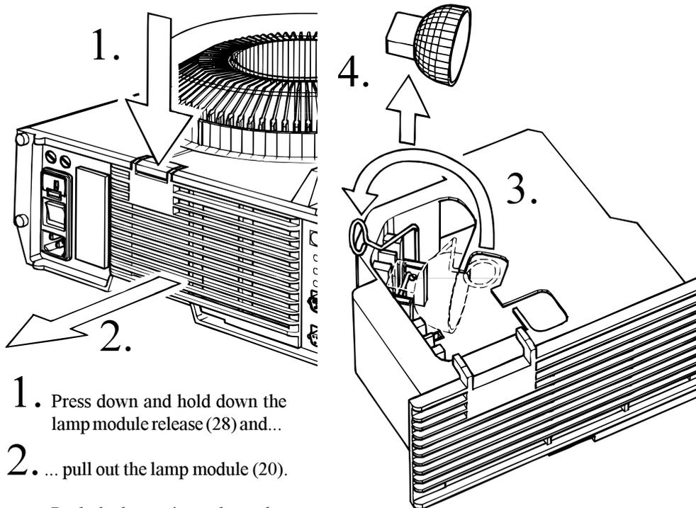
1. Press down and hold down the lamp module release (28) and...
