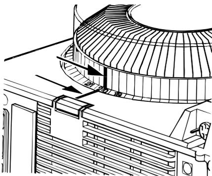
Projectors are often installed on racks where tray installation may be difficult and only possible from the rear of the projector. In this case the tray positioning index mark (27) on the back of the projector is very helpful: The tray is properly set when the index mark aligns with the mark placed on the tray (at slide no. 20 of the 80 slide tray and at slide no. 35 on the 140 slide tray).
