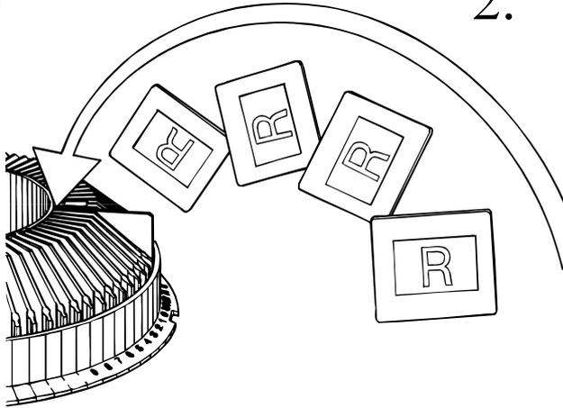
3. Place the loaded tray into its zero position on the projector's transport ring (15). The cleft in the slide tray (zero position) fits on to the notch of the transport ring.
