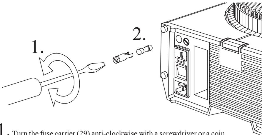
1. Turn the fuse carrier (29) anti-clockwise with a screwdriver or a coin.
