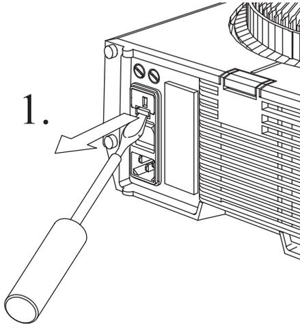
1. Pull out the fuse link compartment (31). Do not change the position of the fuse holder when reinserting into the projector (see also page 26).
