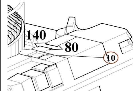
Round trays for both 80 slides and 140 slides can be used. The tray setting switch (10) is set in the factory to accommodate the 80 tray. By using a small screwdriver, the switch can be brought into the 140 position.
