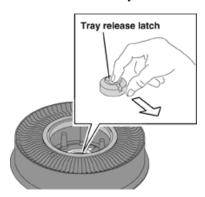
Rotate the metal plate on the bottom of the tray until it locks into position. (For a 140-slide tray, see "Loading the Slide Tray" on page 6.) Put the tray aside.
