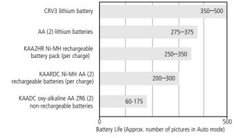
Battery life test method: CIPA (Camera & Imaging Products Association) Memory card used in test: Kodak xD-Picture Card 128 MB
