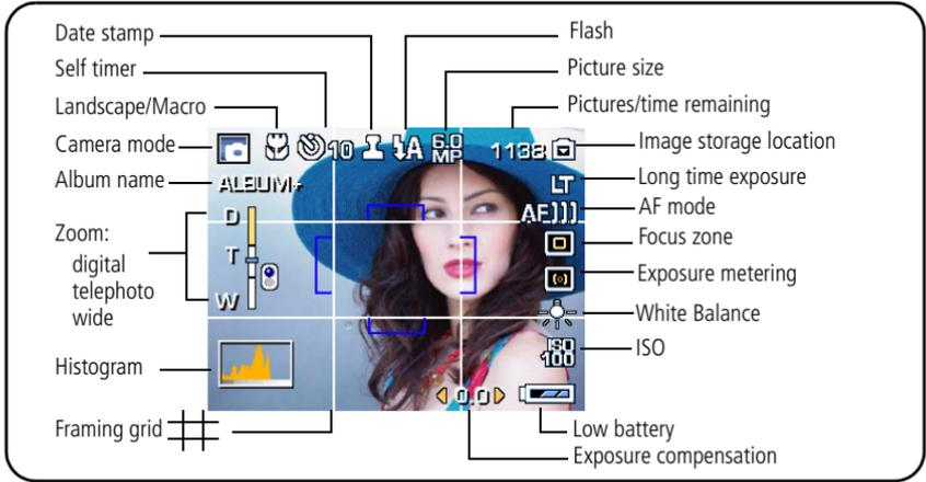
In capture mode—shutter button pressed halfway
