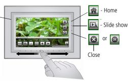
NOTE: When screen icons appear, LEDs turn on at touch-sensitive points along the raised guide.
