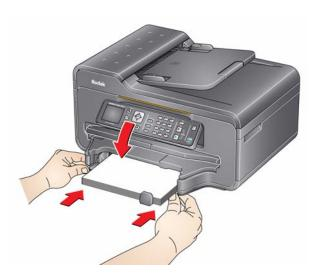
8. Pull out the output tray extender until it is fully extended, but do not lift the paper stop.
