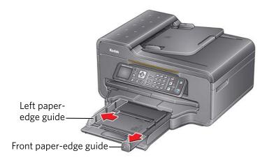
5. Fan and stack the photo paper, then insert the paper (short side first) into the tray with the **logo side facing up** and the glossy side down.
