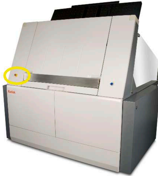
Figure 25: Location of the exterior emergency stop button
