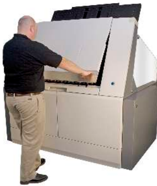
Figure 10: Opening the plate bay door to load plates during normal operation
