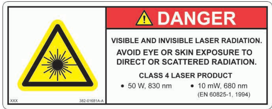
Figure 31: Laser danger label with laser classification and specifications
