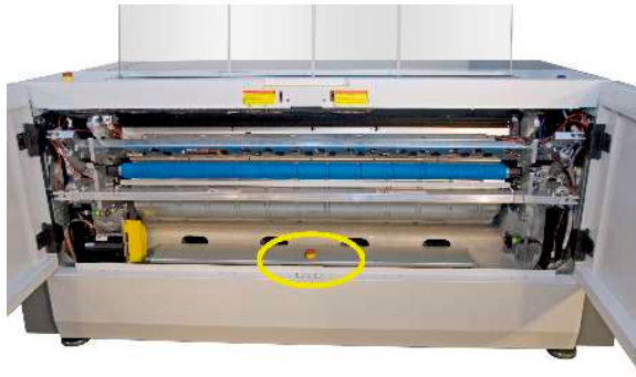
Figure 26: Location of the interior emergency stop button
