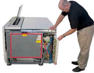
Figure 19: Metal barrier behind right-side panel
