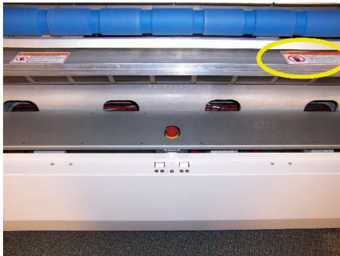
Figure 37: Location of the keep-hands-out label on the leading-edge clamp behind the front panels
