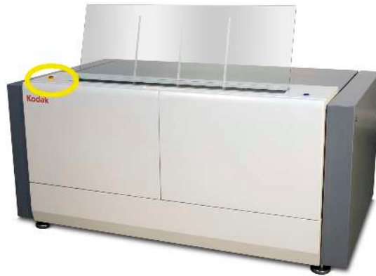
Figure 23: Location of the exterior emergency stop button
