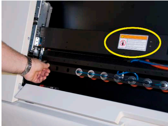
Figure 40: Location of the beware-of-moving-parts label on the picker assembly of the autoloader option
