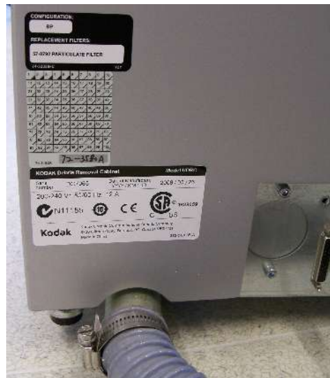
Figure 16: Location of dataplate and configuration labels (shown on a UDRC without external venting )
