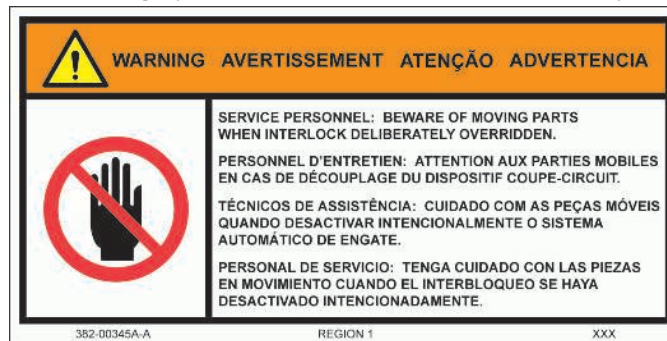
Figure 38: Beware-of-moving-parts label for service representatives
