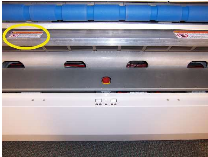
Figure 39: Location of the beware-of-moving-parts label on the leading-edge clamp
