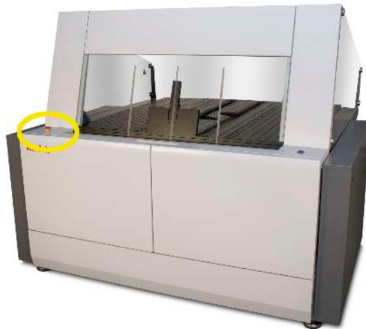
Figure 24: Location of the exterior emergency stop button
