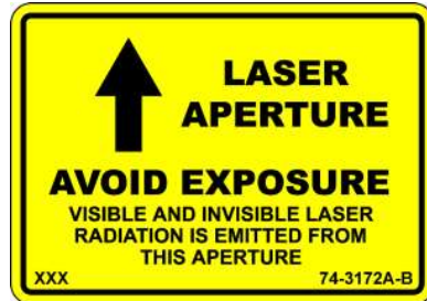
Figure 34: Laser aperture label
