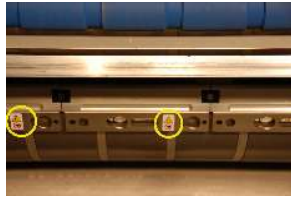
Figure 13: Locations of pacemaker warning labels on trailing-edge clamps
